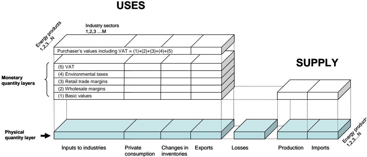
Figure 2. Composition of energy accounts including the relationship between the physical and monetary layers (Olsen, 2007).
